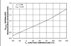
Figure 3. On-Resistance Variation with Temperature.
