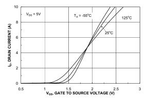
Figure 5. Transfer Characteristics.
