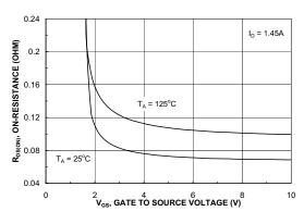
Figure 4. On-Resistance Variation with Gate-to-Source Voltage.
